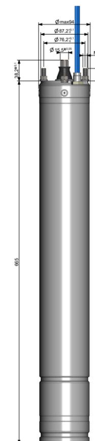
**MOTORI SOMMERSI 4" CON INVERTER INTEGRATO A BORDO, ALIMENTATI DA ENERGIA SOLARE**
